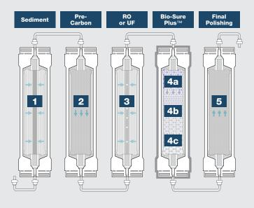
**Sediment Filter** Reduces particles such as dirt, silt, rust and pipe residue. 2 Pre-Carbon Filter Reduces chlorine, chemicals and pesticides. 3 Reverse Osmosis (RO) or Ultra Filtration (UF) Membrane Reduces solids, arsenic, bacteria, viruses, pharmaceuticals, and metals. 4 BIO-SURE PLUS™ FILTER 4a Restores/Adds Minerals & Electrolytes More than 20 minerals and electrolytes are added. **Enhances Alkalinity**
